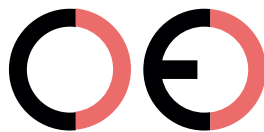
False CE Mark (too far)
